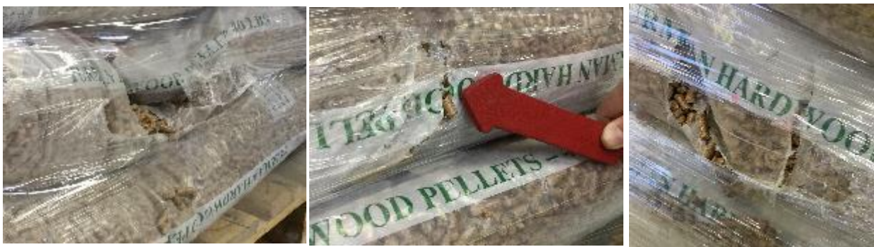
Figure 16 Representative damages of the plastic bags after the pendulum impact test with the SUMO Glove protected fork tine. The average kinetic energy causing failure was 361.70 lb-ft.
