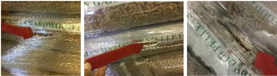
Figure 15 Representative damages of the plastic bags after the pendulum impact test with the sharp fork tine. The average kinetic energy causing failure was 36.17 lb-ft.
