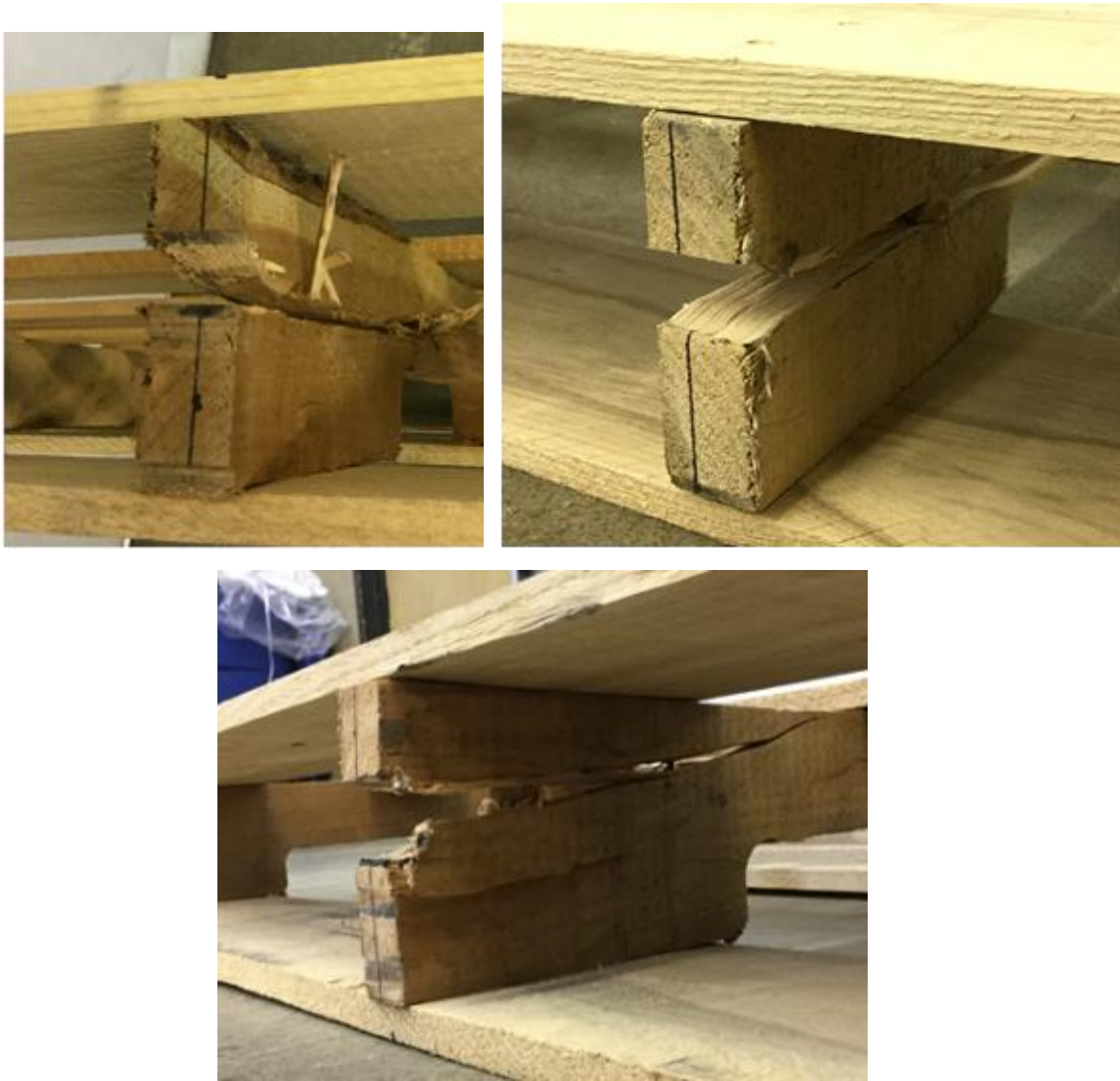
Figure 8 Representative mode of failure of the middle pallet block on the 40 in. end of the investigated wood pallet design when impacted by during sharp fork tines.
