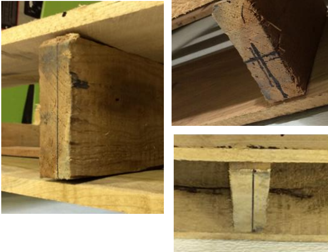
Figure 9 Representative mode of failure of the middle pallet block on the 40 in. end of the investigated wood pallet design when impacted by during SUMO Glove protected fork tines.
