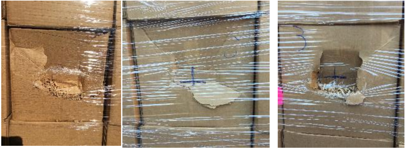
Figure 14 Representative damages of the corrugated boxes after the pendulum impact test with the SUMO Glove protected fork tine. The average kinetic energy causing failure was 140.90 lb-ft.
