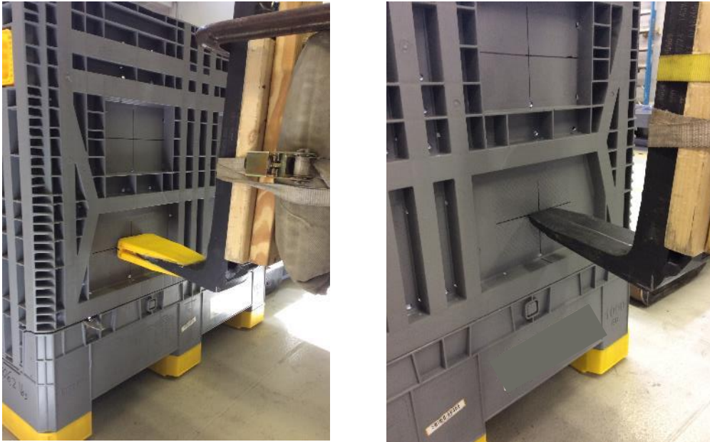
Figure 3 Experimental setup for pendulum impact test of the bulk container using fork tines with and without the SUMO Glove.
