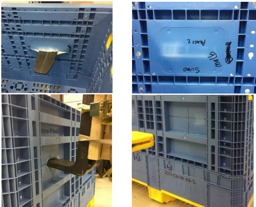
Figure 7 Representative damages of the ISO Bin after the impact with the (left) sharp fork tines and the (right) impact using the SUMO gloves protected fork tines.
